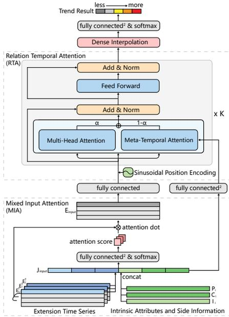
Figure 6: The structure of of attention-based network.
